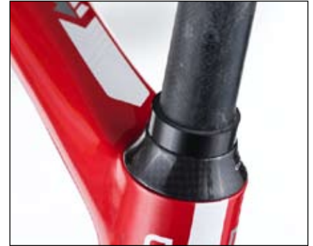
Figure 10. The bearing cover and one spacer on the steerer
